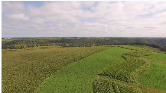
Figure 4. Contour hay strip and grassed waterways in Bridge Creek Watershed.
