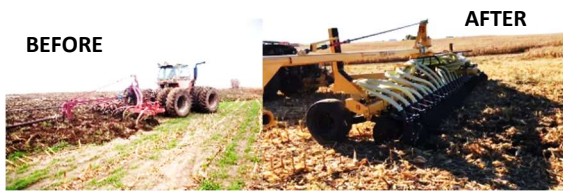
Figure 3. Before 2020 at Field 4- manure injection using high soil disturbance equipment. After 2020- low soil disturbance manure injection system.
