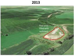
The black and white picture above shows the E3 structure one year after construction in 1955. The adjacent picture, taken fifty-seven years later, shows the four-acre pool area filled with topsoil. This sediment reduced the capacity of this structure to trap additional sediment and nutrients.
