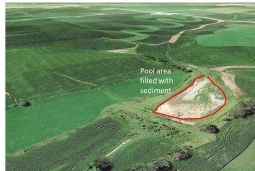
The black and white picture above shows the E3 structure one year after construction in 1955. The adjacent picture, taken fifty-seven years later, shows the four-acre pool area filled with topsoil. This sediment reduced the capacity of this structure to trap additional sediment and nutrients.
