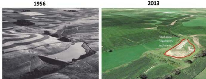
The black and white picture above shows the E3 structure one year after construction in 1955. The adjacent picture was taken fifty-seven years later and shows the four-acre pool area filled with topsoil and much less capacity to trap additional sediment and nutrients.
